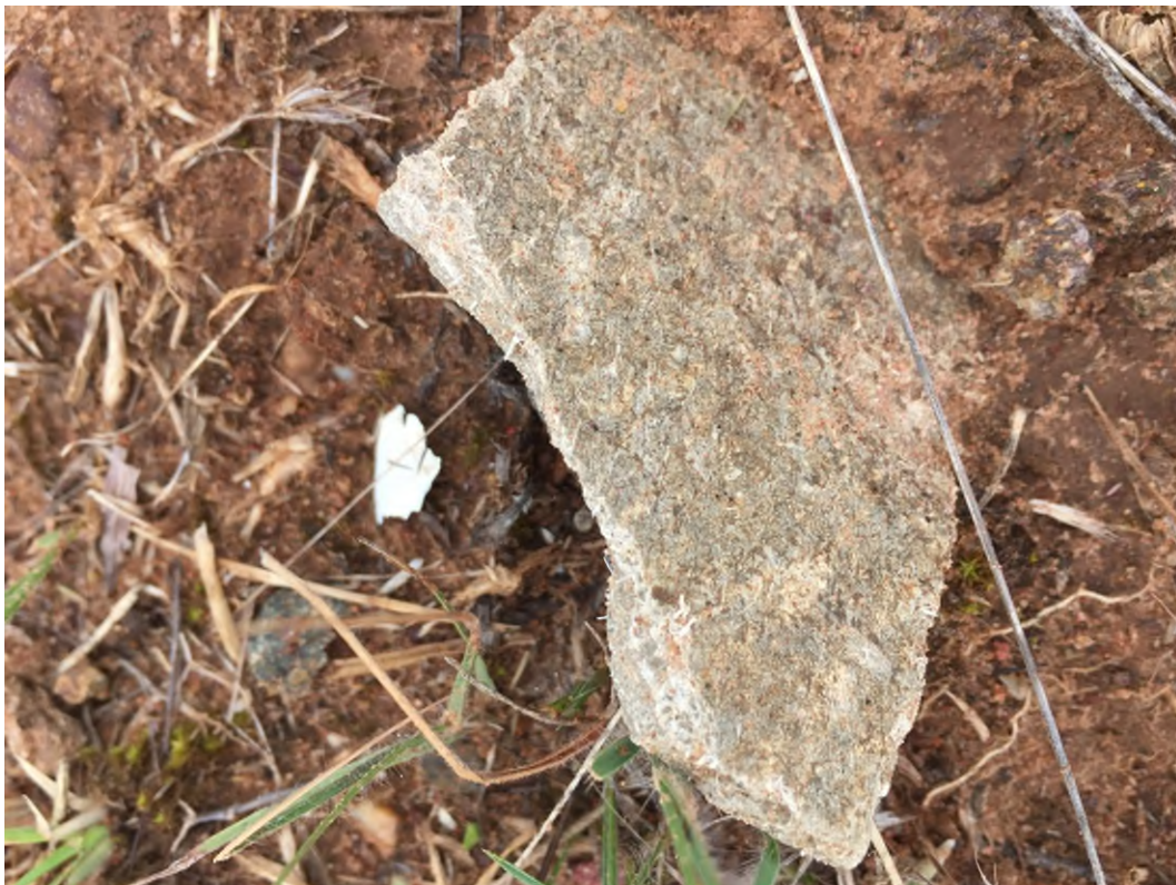
Photograph 8: Close up of non friable ACM fragment in soil.
