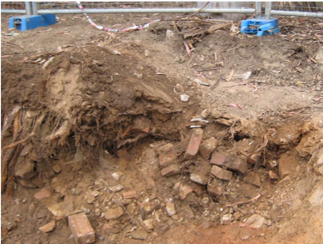
Photograph 5: Example building/demolition rubble in soil.
