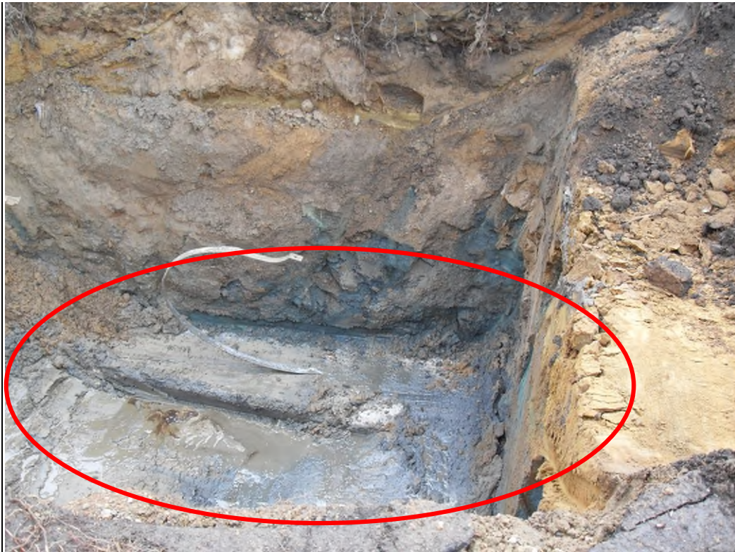
Photograph 3: Example of oily texture due to hydrocarbon products.
