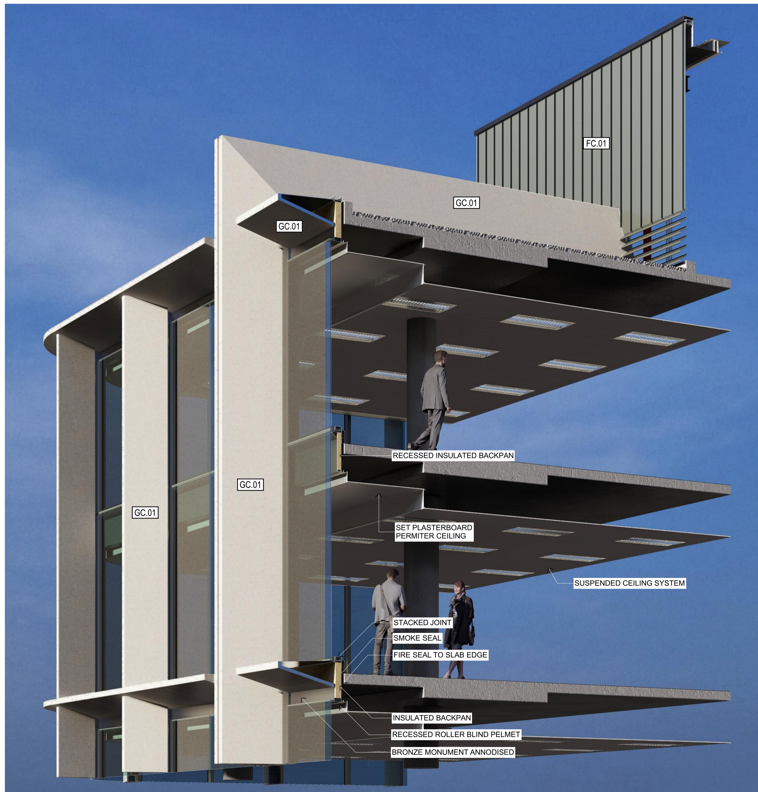
Facade Roof Render Section
