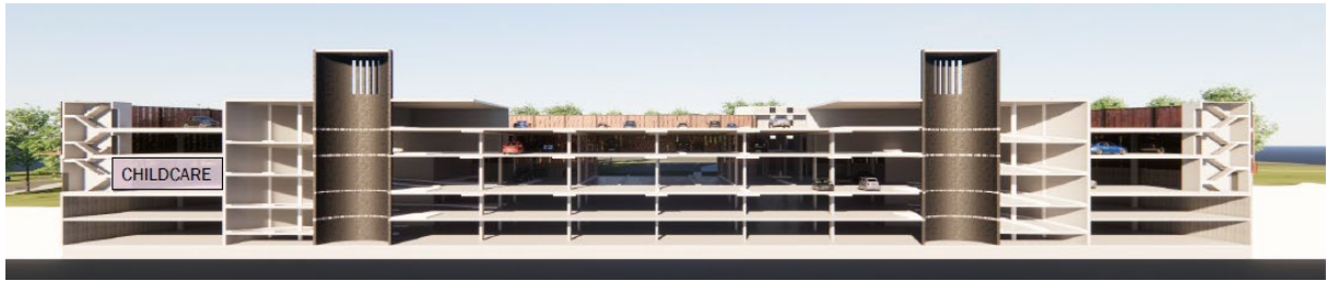
Figure 3.26 Section view of oblong/lozenge design option for carpark and including two basement levels. (Source: BVN 21 July 2021)
