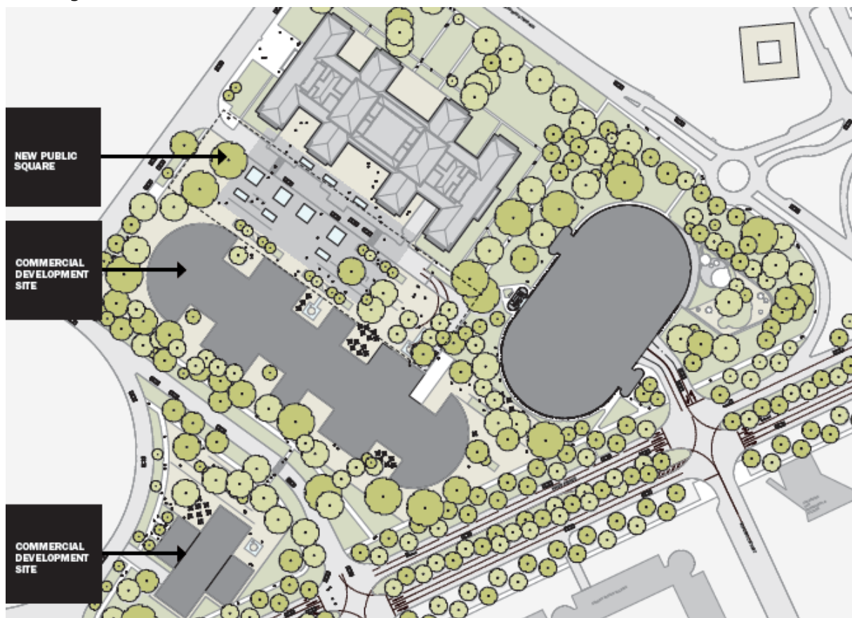
Figure 3.23 Proposed final masterplan with the carpark located in the northeast corner of the site and a potential future core function building to the southwest completing the 'campus'. (NB: design shows an earlier 'oblong'-shaped proposal for carpark structure). (Source: BVN Design Report, 2 November 2021, p 116.)
