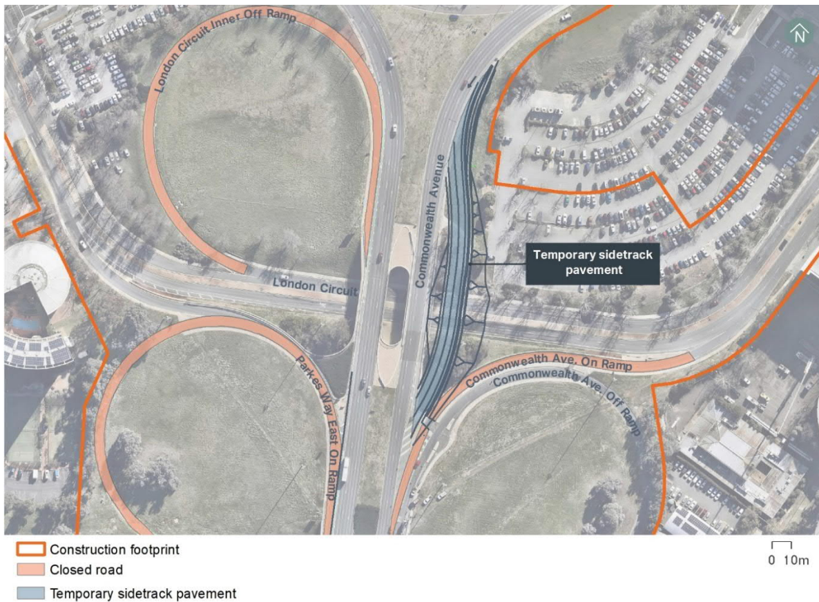
Figure 5 Temporary Commonwealth Avenue sidetrack configuration
