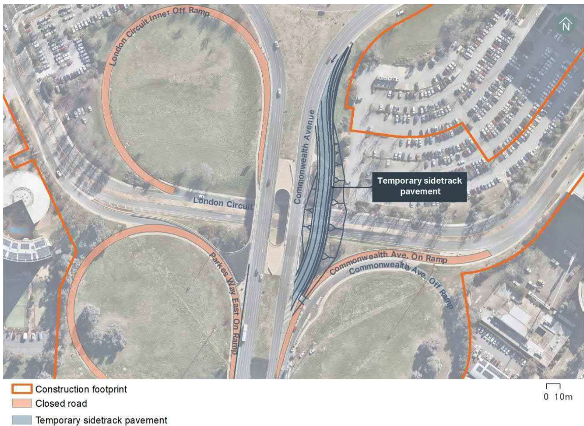
Figure 2-3 Temporary Commonwealth Avenue sidetrack configuration
