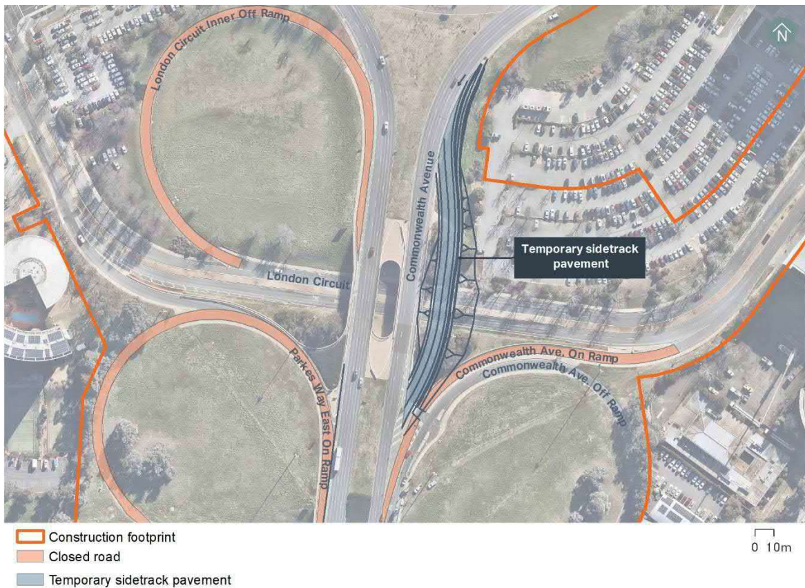
Figure 2-3 Temporary Commonwealth Avenue sidetrack configuration
