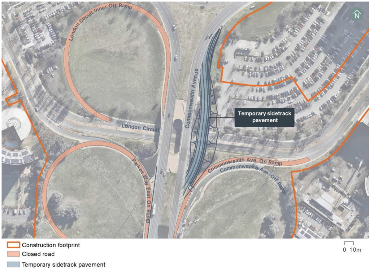
Figure 2-3 Temporary Commonwealth Avenue sidetrack configuration
