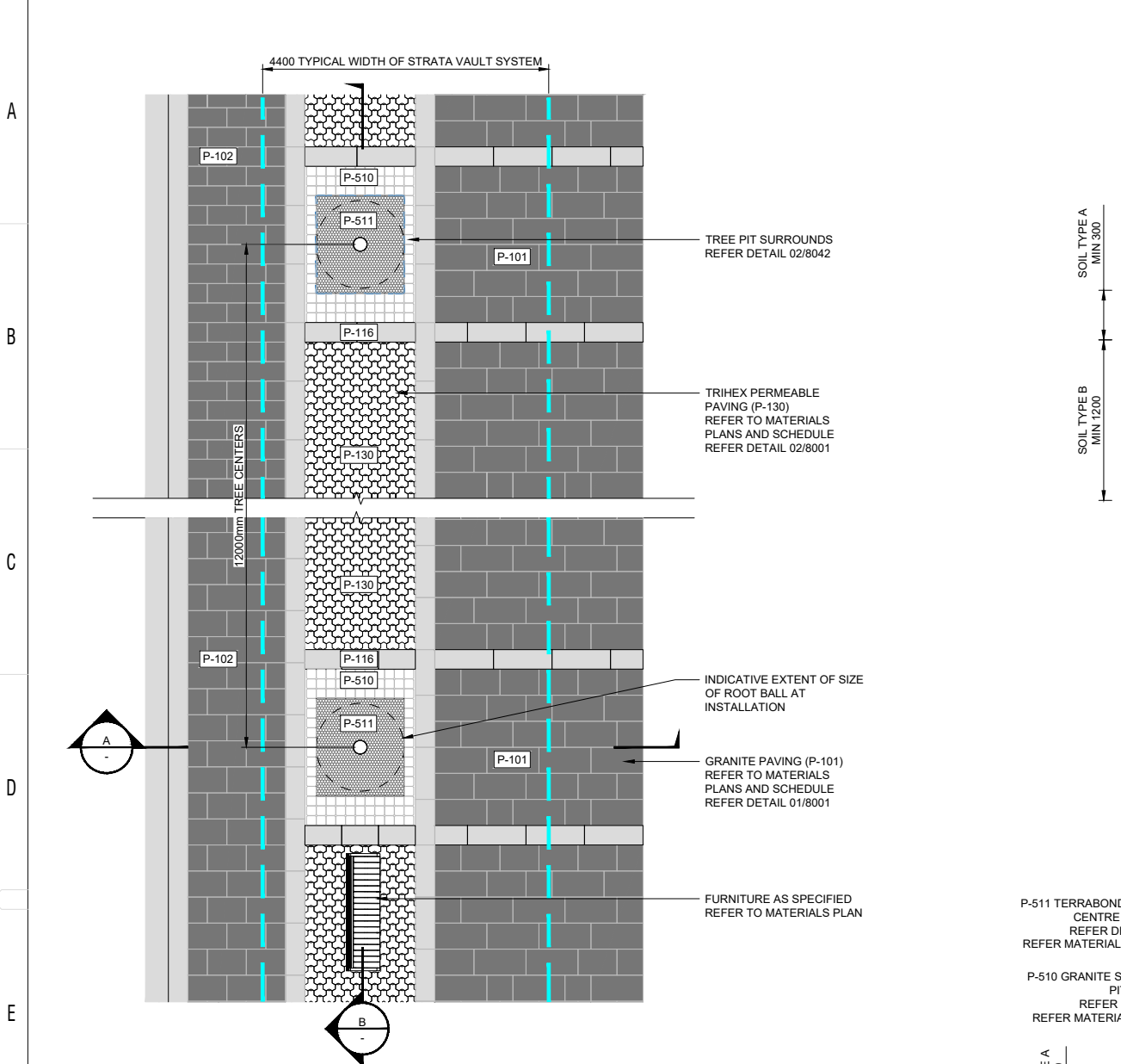
A | TYPICAL TREE PLANTING WITH STRATA VAULT - SECTION SCALE 1:25
