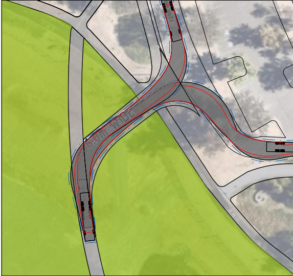
EMERGENCY SERVICE ACCESS TURNING MOVEMENT - 12.5m VEHICLE
