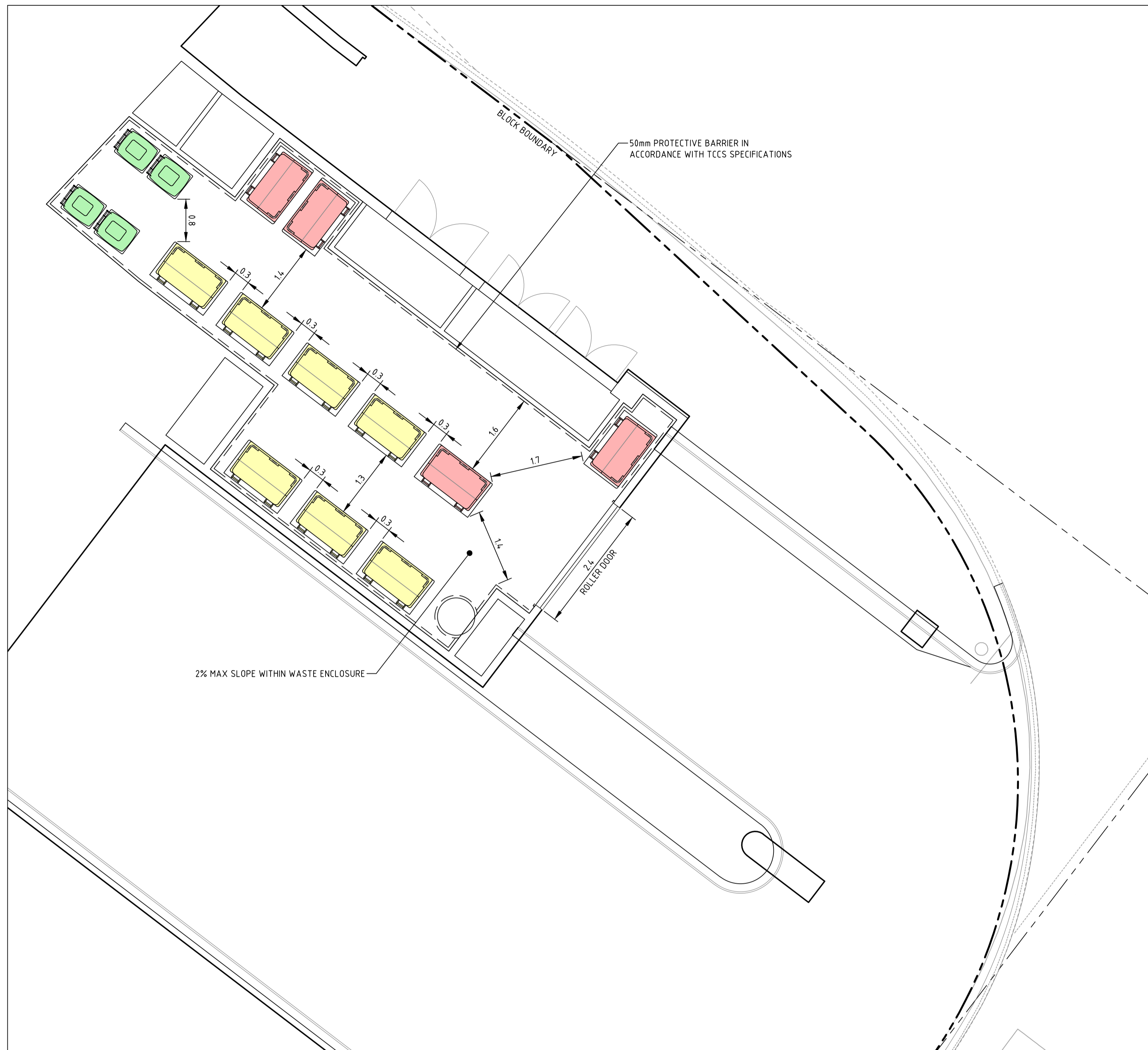
DETAIL A WASTE ENCLOSURE SCALE 1:50
