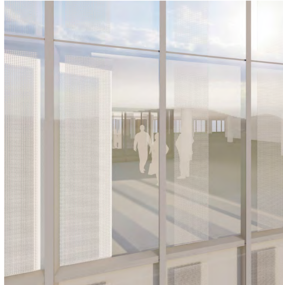
APPLIED FRIT SOLAR CONTROL TO GLAZING
