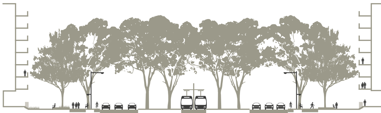
FIGURE 11 FORMAL LANDSCAPE AVENUE CROSS-SECTION MEDIUM TERM NORTHBOURNE AVENUE 3 LANES EACH WAY WITH SEPARATE CYCLE LANE
