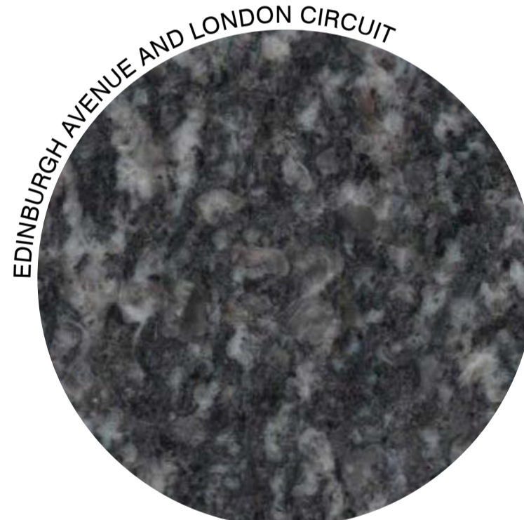
Paving Type 3 Kimberley Storm granite paving 400 x 600mm
