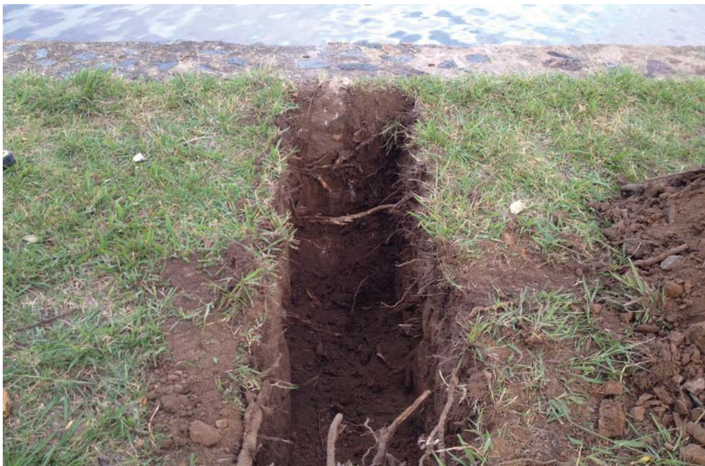
Photo 6 – View of front of Test Pit 2 adjacent to the lake wall
