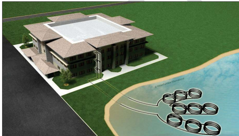
Figure 4: Closed Water Loop.
