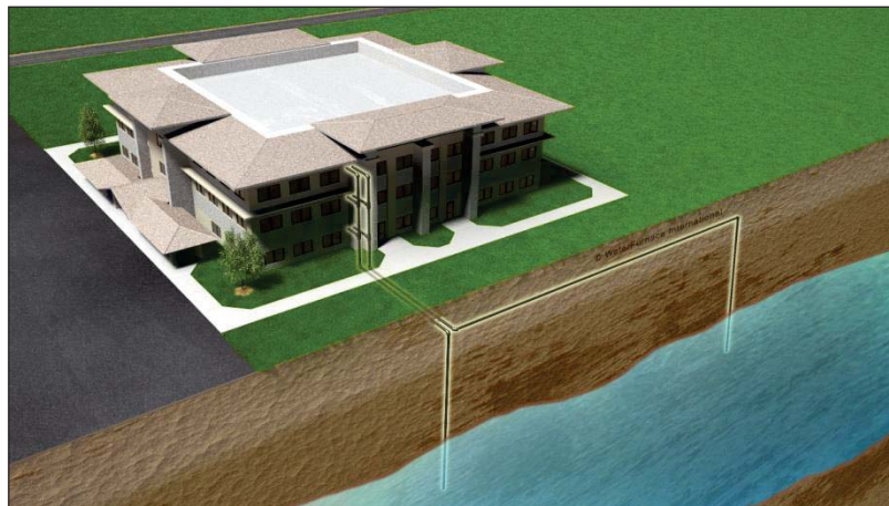
Figure 5: Open Groundwater Loop.
