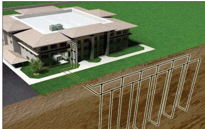
Figure 6: Vertical ground loop with ‘fluid cooler’ hybrid.
